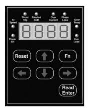
MOTOR FLA (F001) must be programmed for unit to operate! Display Shows...
